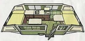
Romada Specifications: Weight, 1740 lbs.\* \* Length, 16'61/2" . Width, 6'77/8" . Road Height, 53" . Tires, 20.5x8.0-10", 6-ply-rated. Living Area: Height, 6'2" . Width, 6'51/2" . Length, 20'7" . Bed Dimensions, 72" x 54".
